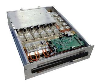
Compact design technology allows 6kW output power contained in each amplifier module, with up to 8 modules in the same rack
