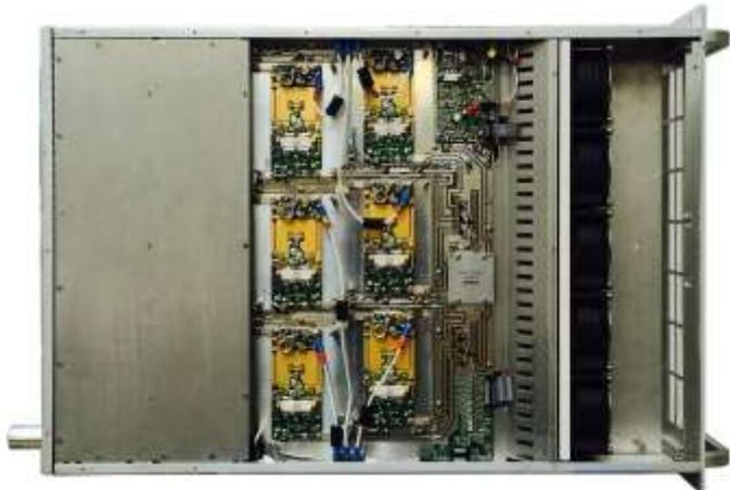
*Compact design technology allows 5kW output power with exciter built-in contained in only 19" drawer four rack units*
