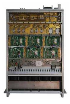
Compact design technology allows 5kW output power amplifier in only 19" drawer four units high with 3 AC/DC switching power supplies and 6 RF block of 1,2kW each
