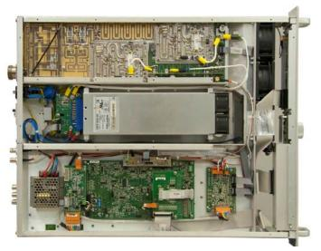
Very compact design technology allows 2kW output power with exciter built-in contained in only 19" drawer two units high.
