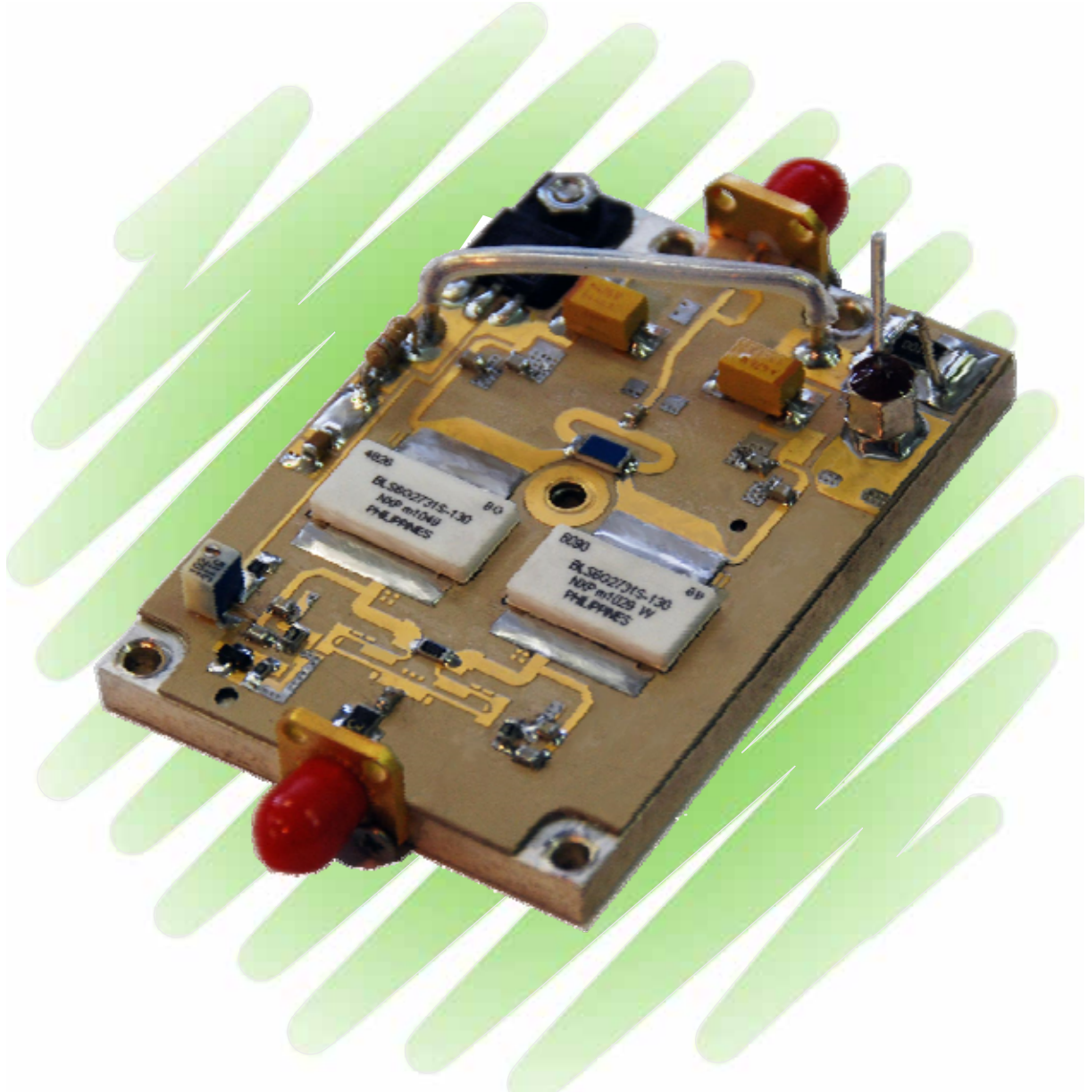
250W S-Band Pulsed Amplifier
