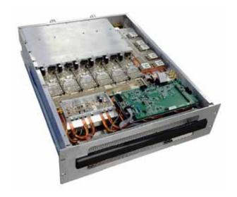
Compact design technology allows 5,5kW output power amplifiers in only 19" drawer three units height combining 6 RF blocks of 1 kW CW each, with the relevant pre driver section.
