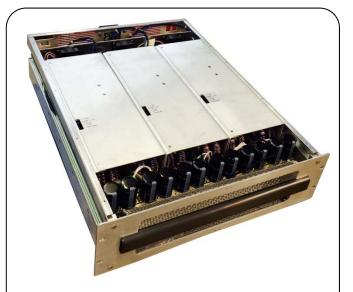
The 19" drawer also accommodates three AC/DC switching power supplies capable of 3,5 kW each, and the relevant capacitors bank section for optimal pulsed operation capability.
