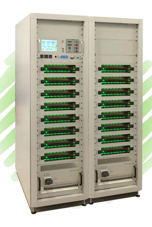
80 kW CW , 81.25 MHz SSPA LIQUID COOLED
