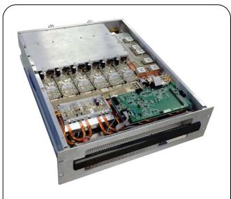
Compact design technology allows 5,5 kW output power amplifiers in a 19" drawer, three units height , by combining 6 RF blocks of 1,2 kW CW each , along with the relevant pre driver section.
