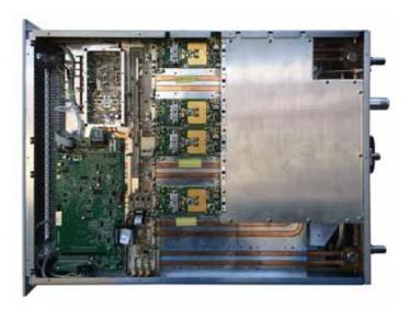
Compact design technology allows 4,0kW output power amplifiers in only 19" drawer three units height combining 4 RF blocks of 1,2 kW CW each, with the relevant pre driver section.
