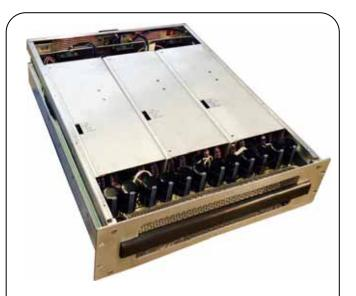
The 19" drawer three units height also accommodates 3 AC/DC switching power supplies capable of 3,5kW each, and the relevant capacitors bank section or optimal pulsed operation capability.
