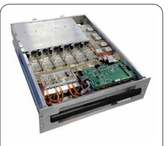
Compact design technology allows 5,5kW output power amplifiers in only 19" drawer three units height combining 6 RF blocks of 1,2 kW CW each , with the relevant pre driver section.
