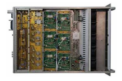
Compact design technology allows 5kW output power contained in only 19" drawer four rack units
