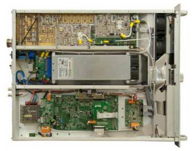
Very compact design technology allows 2kW output power contained in only 19" drawer two units high.
